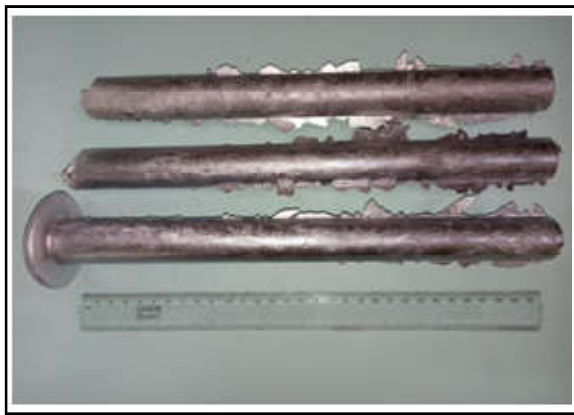
Fig.2 As-cast specimen (Stir Casting)
