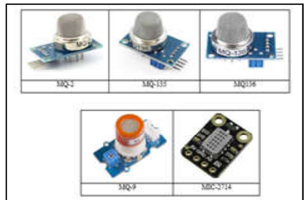
Fig.6 Gas Sensors of Hexacopter for air quality surveillance
