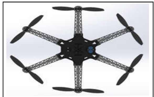
Fig.3 Design of Arm and Propeller design – Hexacopter
