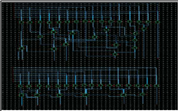
Fig.4 Schematic of 4*4-bit Vedic Multiplier in cadence tool
